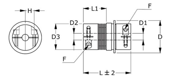
D = 109Nom. torque NM (Tkn) = 90NM overload torque range 1 Position engagement = C = SynchronousD1 = 25
